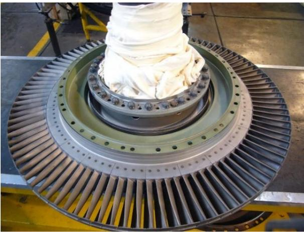
**Figura 1** Rotor de turbina FT - 4C1 Pratt & Whitney [1.1]
